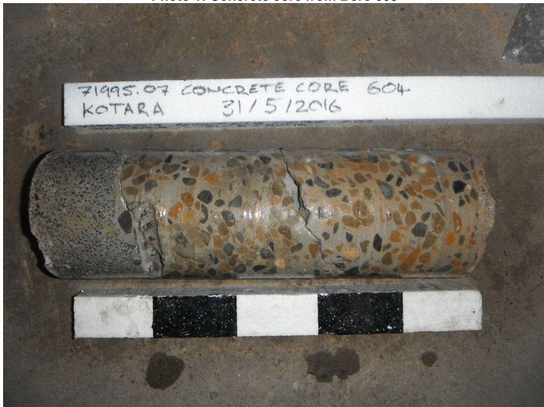
Photo 2: Concrete core from Bore 604
