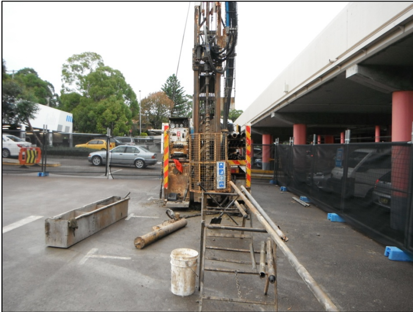
Figure 12: Truck mounted drilling rig at Bore 107
