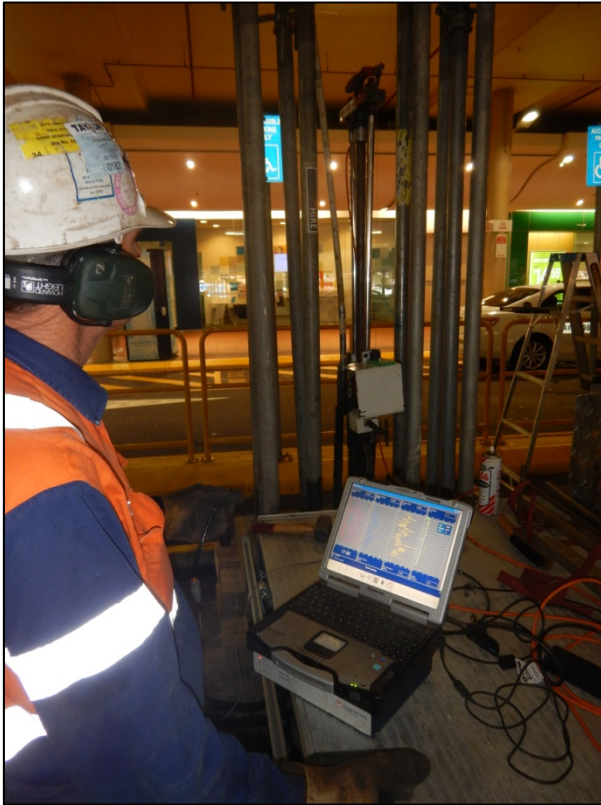
Figure 11: Capture of CPT investigation data
