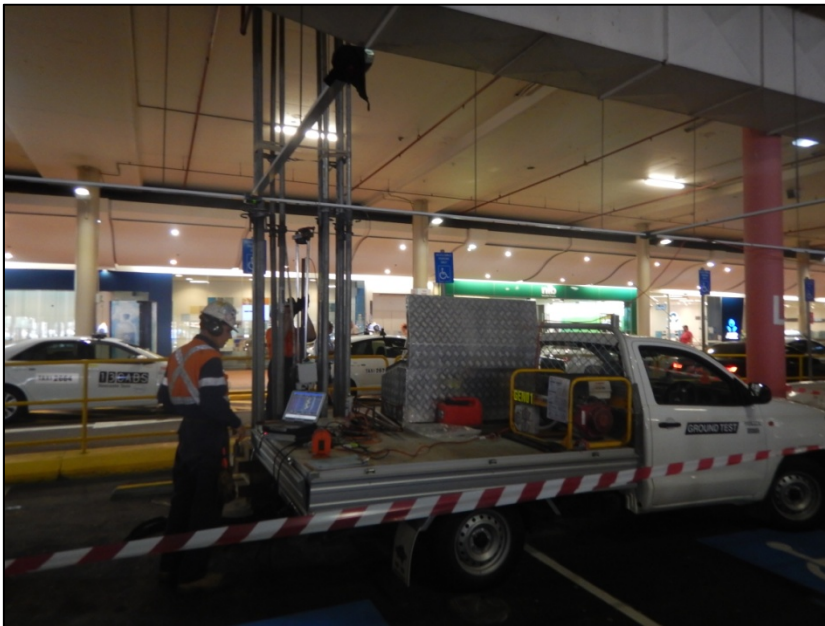
Figure 10: Typical set up of portable CPT equipment
